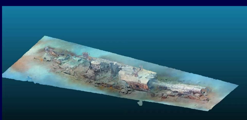
3D geo-reconstruction from still photo survey Fully automated process from ~4000 images
